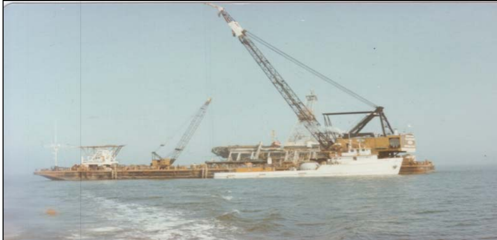
Figure 5.1. Kerr McGee Rig 39, the Frank Phillips, with a Drilling Tender and Converted Navy YF Barge. Photo Courtesy of Chester Pipsair, OOGHP.
