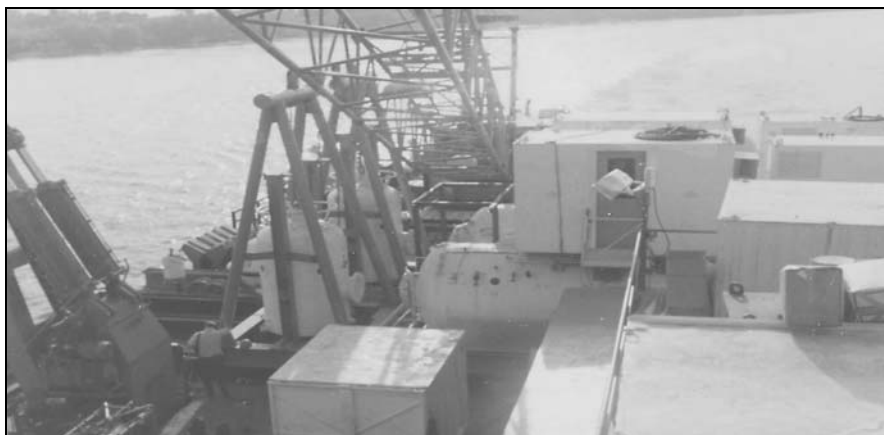
Figure 6.14. Saturation Diving Spread on the Back of a Barge; Decompression Chamber in Center, Control Van on Top, Bell on Left, 1969. Photo Courtesy of Drew Michel, OOGHP.
